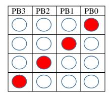
Once PB3 is on the next output should go back to PB0 being on. There should be a 300ms delay between each step. The program should repeat indefinitely. All outputs should be sent one at a time. Use an 8 bit (char) array to hold the values to be sent the port.
