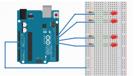
[We will use a  $220\Omega$  sip for the resistors shown above (the common pin of the sip will go to ground]
