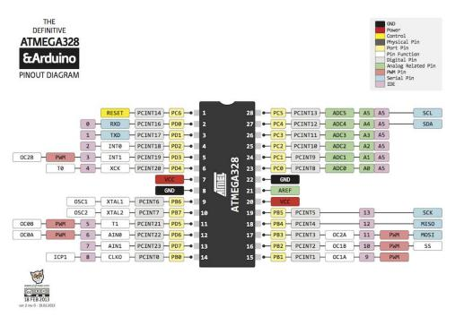
Remember that Arduino pins and Atmega pins are NOT the same. PB0 is on the IC on pin 14 but on the Arduino headers it is IO Pin 8 (for example).
