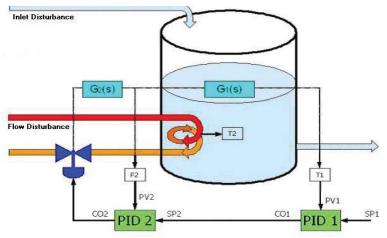
In this example of cascaded PID control of tank outlet temperature, PID 1 can be referred to as Master, Primary, or Outer Loop; PID 2 can be referred to as Slave, Secondary, or Inner Loop.
