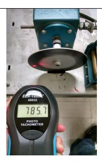
Hold the Test Button in to obtain reading on LCD display.
