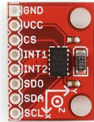
Note: This is a 3.3v device, so like the LCD, you will have to use the Bi-Directional Logic Level Converter to connect the device to the Arduino<sup>1</sup>:
