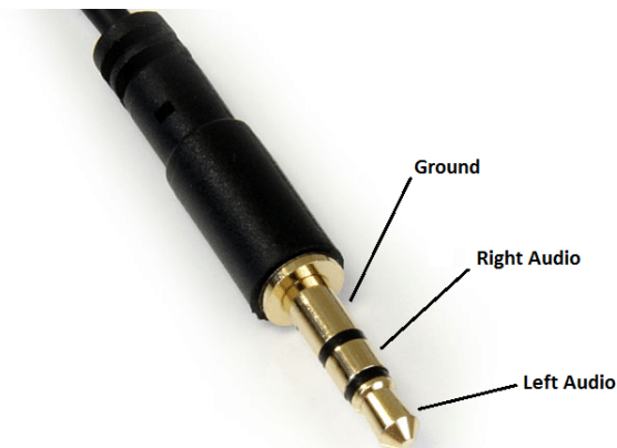
Figure 1 - 3.5mm Jack Connections
