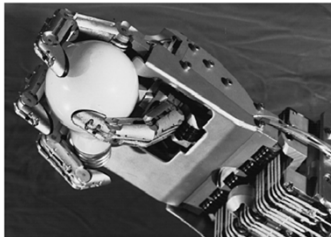
The Utah/MIT Dextrous Robotic Hand: A dextrous robotic hand having 18 degrees of freedom, developed as a research tool by the Center for Engineering Design at the University of Utah and the Artificial Intelligence Laboratory at MIT. It is controlled by five Motorola 68000 microprocessors and actuated by 36 high-performance electropneumatic actuators via high-strength polymeric tendons. The hand has three fingers and a thumb. It uses touch sensors and tendons for control. (Photograph by Michael Mitochik. Courtesy of University of Utah.)
