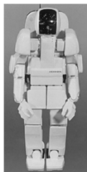
The Honda P3 humanoid robot. P3 walks, climbs stairs and turns corners. Photo courtesy of American Honda Motor, Inc.
