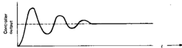
C. Stable - Underdamped
