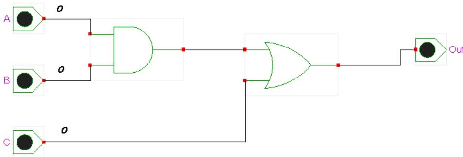
And start working though the circuit to derive the next output. So here, A=0 and B=0, since they are going through an AND gate, the output of the AND is 0, now that 0 and C (which is also zero) go into the OR gate. Since 0 OR 0 is 0 the Output is 0. So for row one, the output is 0.
