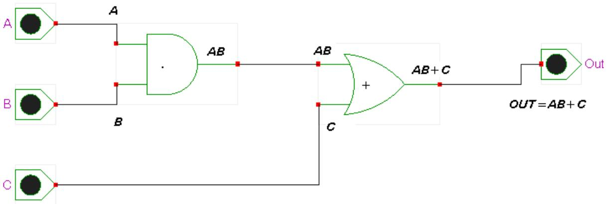
For the Truth Table, First fill in all the possible inputs (using a binary count for the order of inputs AND to insure you cover all possible input combinations). Since there are 3 inputs (A,B,C) you will need three columns. Start the count at 0 decimal or 000 Binary and count all the way to 7 decimal or 111 binary. The table will look like:
